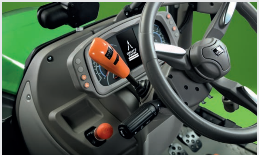
↑ PowerShuttle with SenseClutch (5 adjustable levels).
