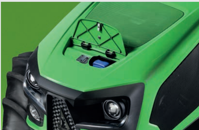
↑ Easily accessible AdBlue tank (not applicable in New Zealand).
