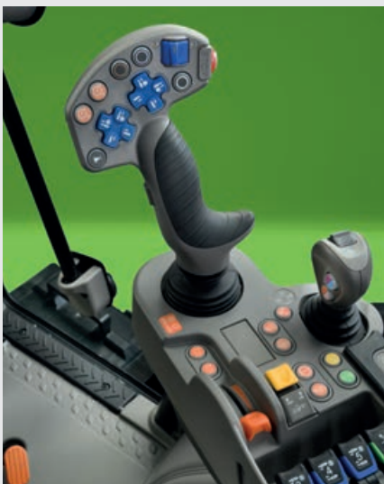
↑ MaxCom Joystick to allow easy management of driving speed.
