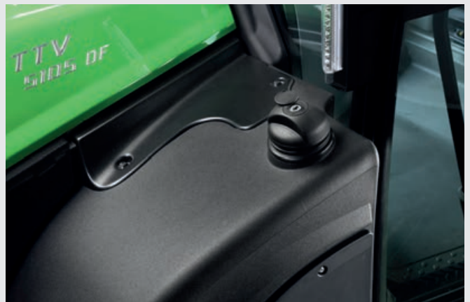
↑ Easy refuelling and long working days are ensured thanks to new fuel tank.
