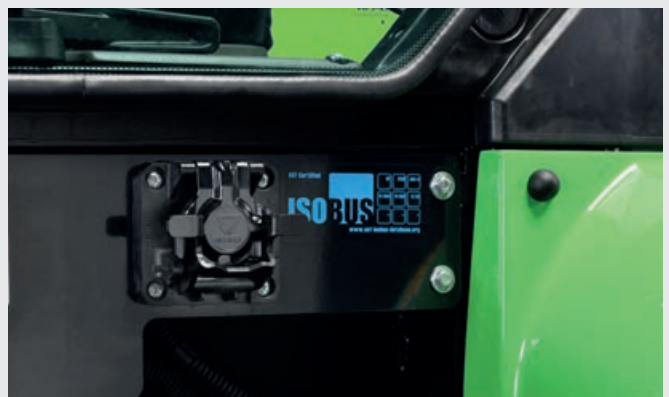
↑ ISOBUS: you can plug any type of implement and benefit from various ISOBUS features.
