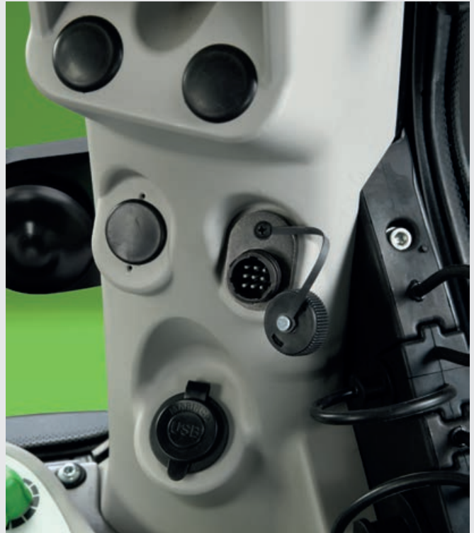
↑ In-cab ISOBUS plug for additional monitors.
