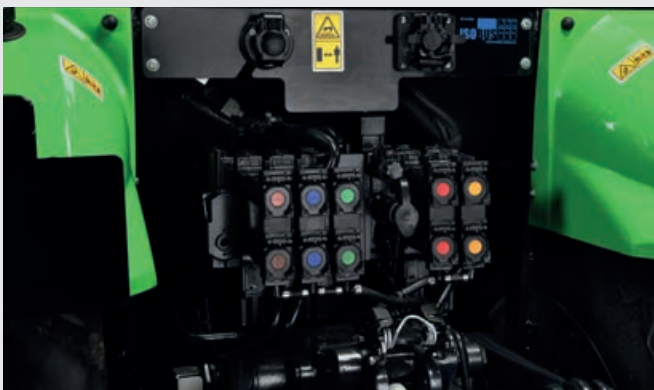
↑ Up to 5 electronically controlled rear distributors.
